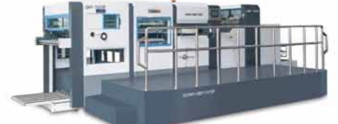
MY-series SEMI-AUTOMATIC DIE-CUTTING & CREASING MACHINE YARI OTOMATİK KARTON - OLUKLU KESİM MAKİNASI
